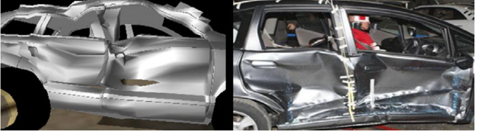
Fig. 3. Left: metal deformed without applying the spring-mass model. Right: Car collision in real world.
